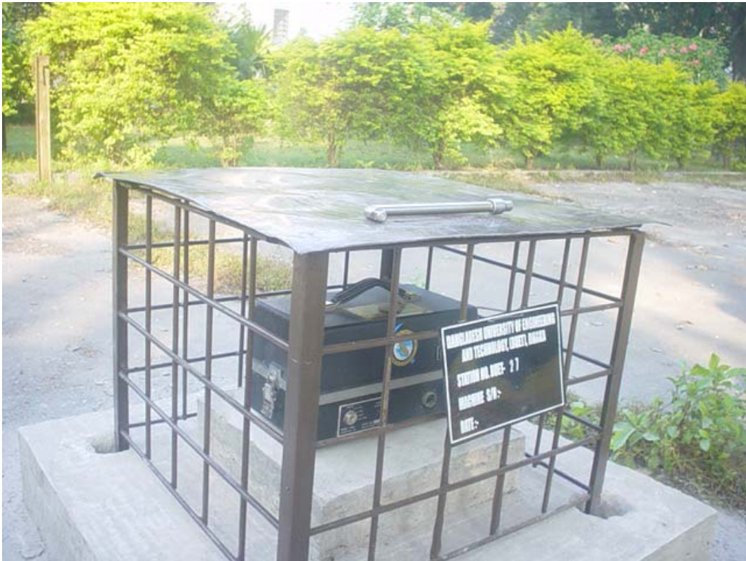
Figure 22. SMA at Gaibandha
