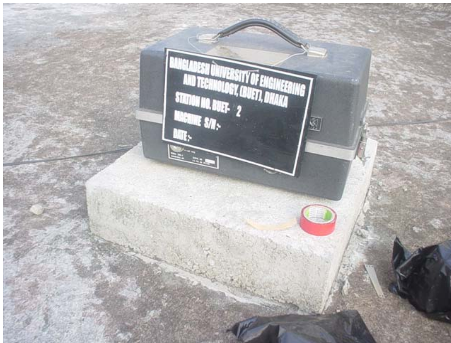
Figure 7. SMA at top floor, Civil Building, BUET
