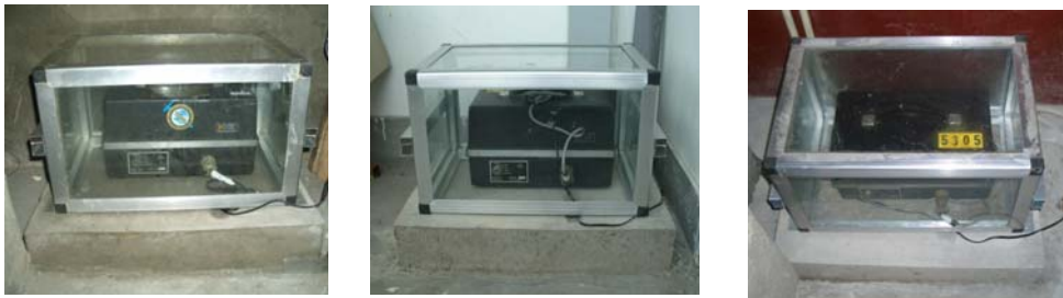
Fig. 5 Some accelerographs installed on different stories in ICC
