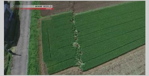
(Above) Lateral ground shifts of up to ~2m were observed along the surface trace of a 50-km fault ruptured by the 15 April 2016 M7.0 earthquake of, in south-western Japan. (Quote and photo from [Earthquake-Report.com](http://Earthquake-Report.com), last accessed 11/12/2016)
